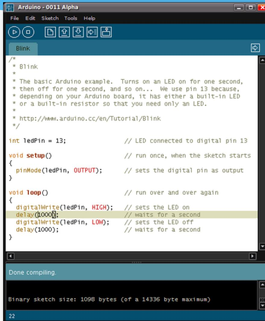
The image shows a screenshot of the Arduino IDE interface. The window title is "Arduino - 0011 Alpha". The menu bar includes "File", "Edit", "Sketch", "Tools", and "Help". The toolbar contains icons for running, stopping, saving, opening, and uploading. The sketch name is "Blink". The code editor displays the following C++ code:
